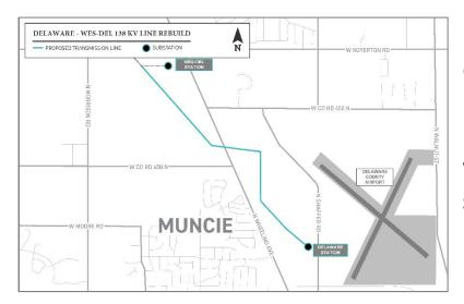
Project Snapshot: Construction Start: Fall 2019 Energized: Winter 2019 Miles: 2.2 Voltage: 138-kV Double-Circuit Structures: 16 Route: Residential, Rural
